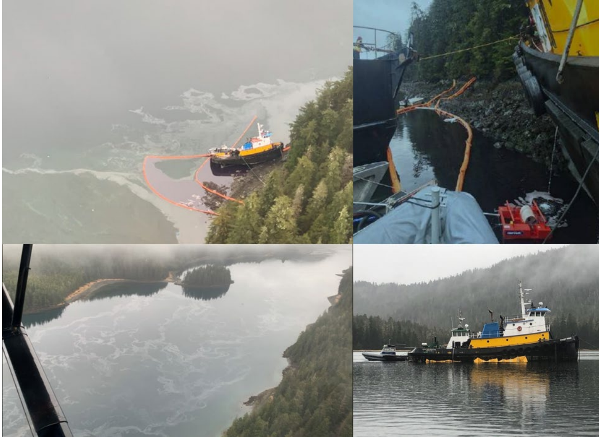
Figure 3: Oil around grounded vessel on the morning of March 23 (top left, photo credit: ADFG); skimmer recovering product inside the containment boom on March 23 (top right, photo credit: Global Diving and Salvage, Inc.); oil sheen in Neva Strait on March 23 (bottom left, photo credit: ADFG); tug Western Mariner afloat in Neva Strait before being towed to Sitka on March 29 (bottom right, photo credit: SEAPRO)
