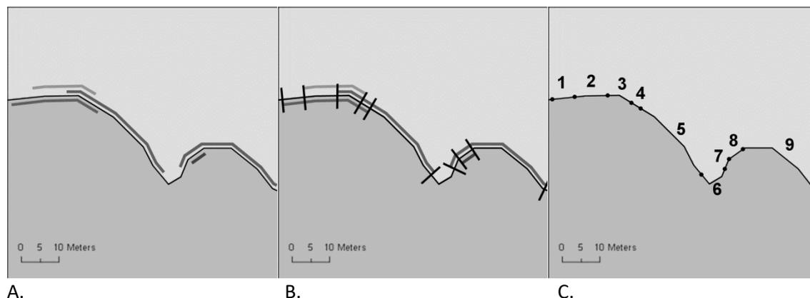
**Figure 2.** Schematic of A.) multiple hypothetical overlapping coincident line segments, B.) those same line segments intersected with themselves and C.) resulting unique line segments formed by overlap of all linear survey observations over time.
