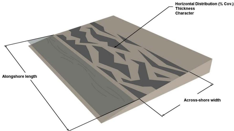
**Figure 1.** Schematic of observational metrics used to describe surface oiling along linear portions of a shoreline.
