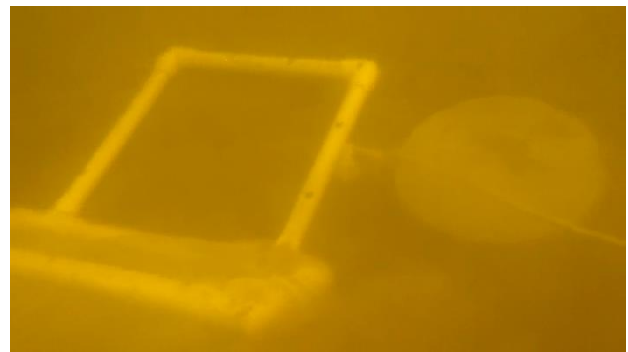
Figure 2: 0.0625 m 2 (0.25 m x 0.25 m) quadrat sampler with 6 mm mesh bag attached placed adjacent to the marker anchor on the river bottom. Sediment is excavated to a depth of ca. 15 cm at two sites (one on each side of the anchor) within the quadrat site for a total sampled area of 0.125 m 2 .
