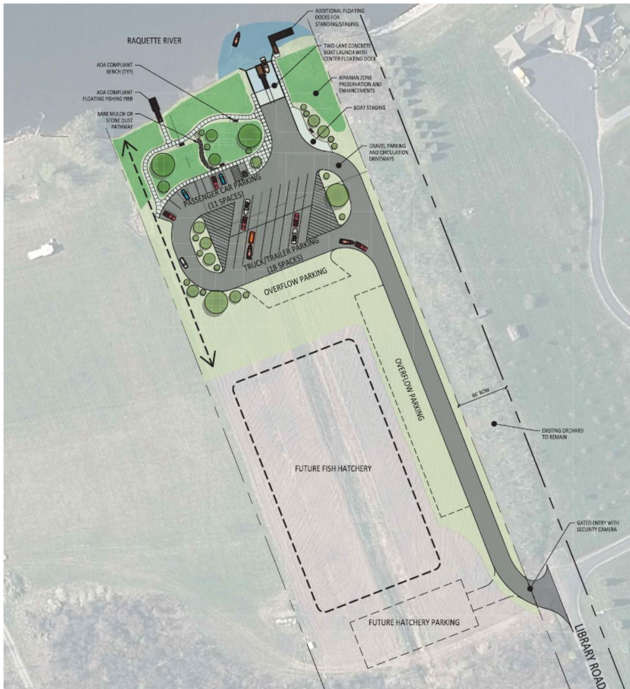
Figure 9. Conceptual plan for the Raquette River Public Access Project (Alternative 1C). Parking lot configuration may change, and potential fish hatchery to be addressed in future planning document.
