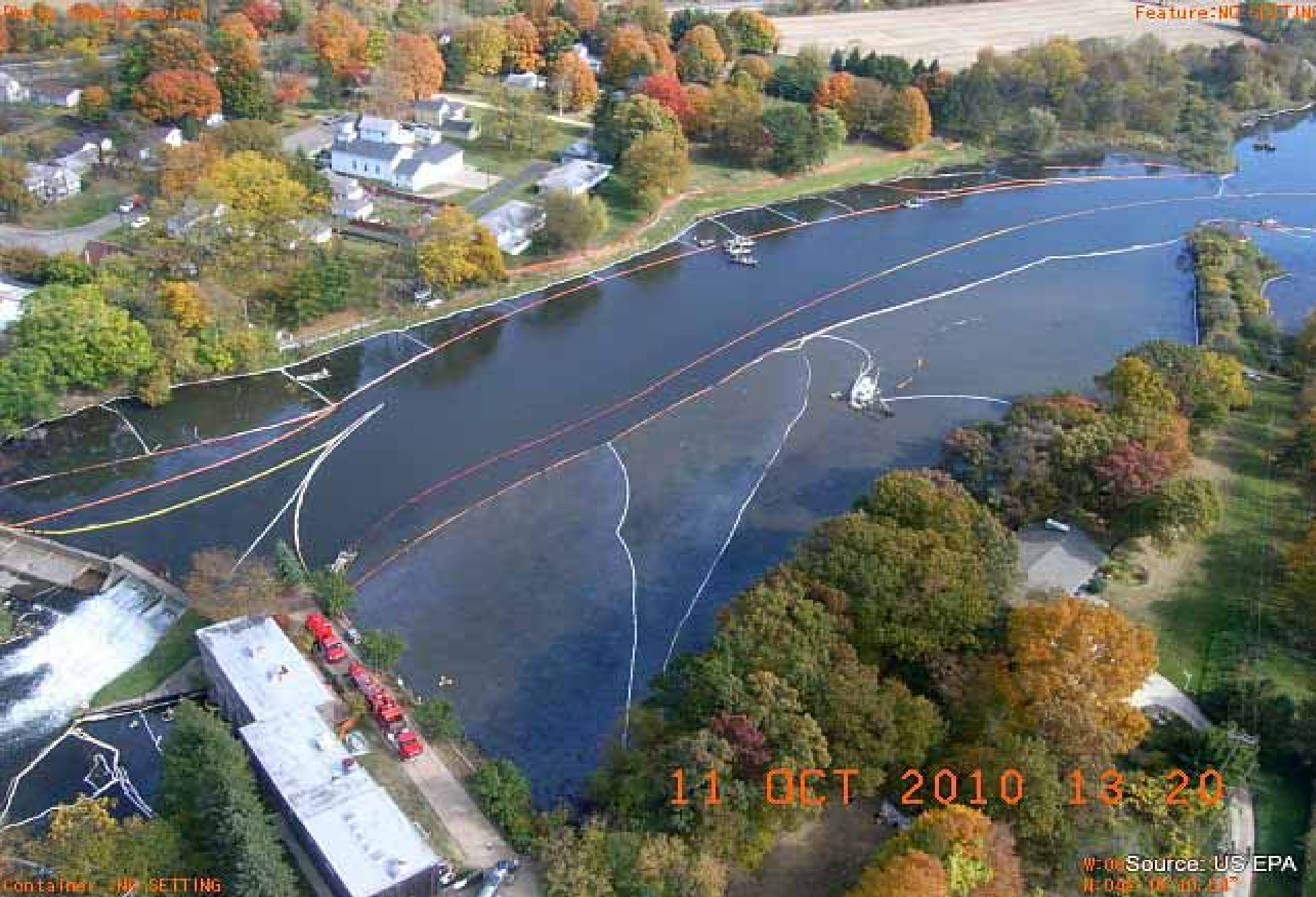
Ceresco Dam dredging operation and submerged oil aeration cells along the north bank.
