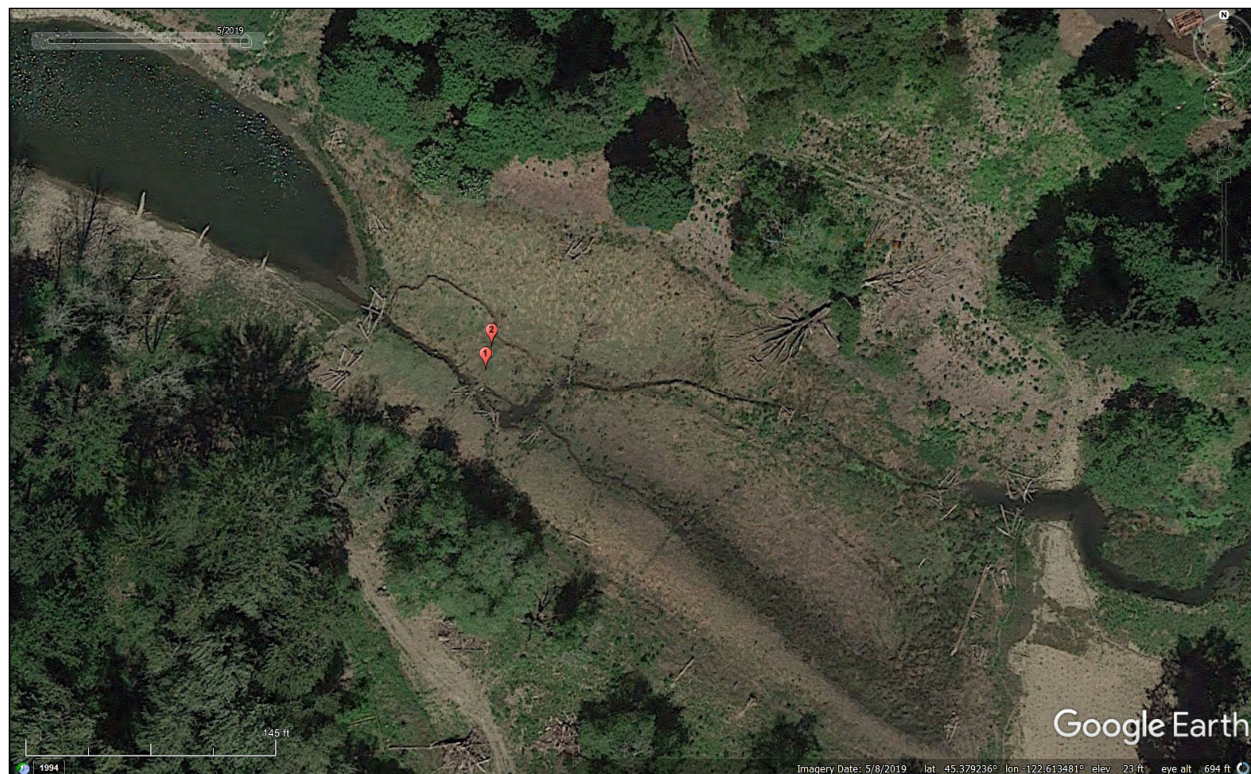
Figure 8 Locations of headcuts #1 and #2 did not change from July 17, 2019, to April 3, 2020. Their vertical height was reduced in size.
