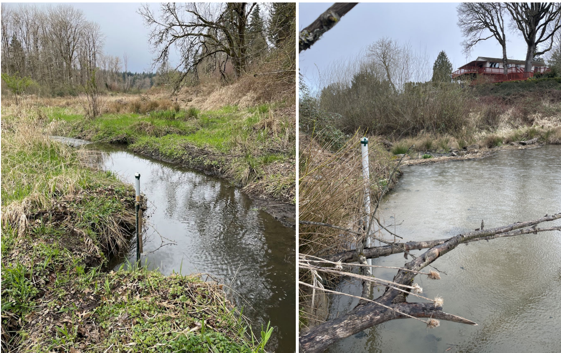
Figure 2-4: Waterways water level loggers installed on site.
