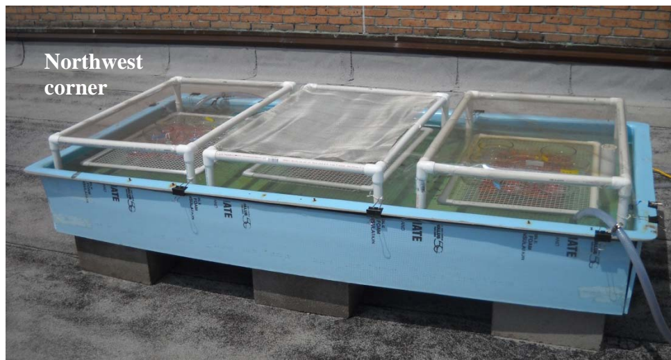
Figure F.1. Water table set-up for UV exposure to embryos.
