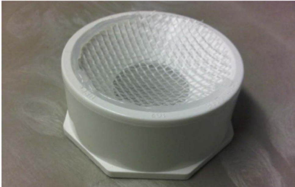
Figure 5.2. Spawning ring for inducing natural spawning in sheepshead minnows.
