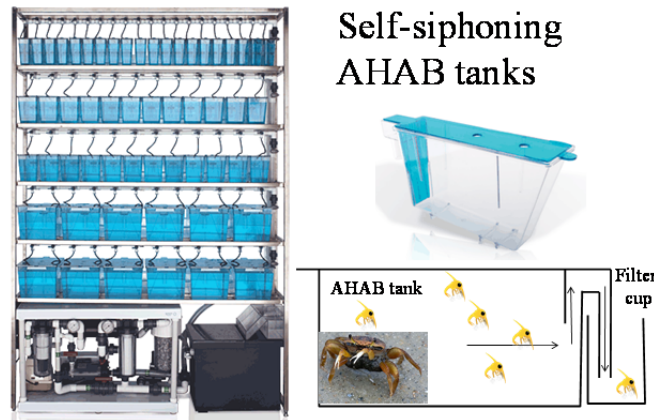
Figure A.2. Recirculating AHAB tank system used to hold gravid females and collect and enumerate fiddler crab larvae. Water first circulates through each tank, and then through biological and mechanical filters to maintain water quality. Each tank drains through a spigot under which collection filter cups can be placed. Gravid females were placed in individual tanks, and filter cups were checked daily for crab larvae.
