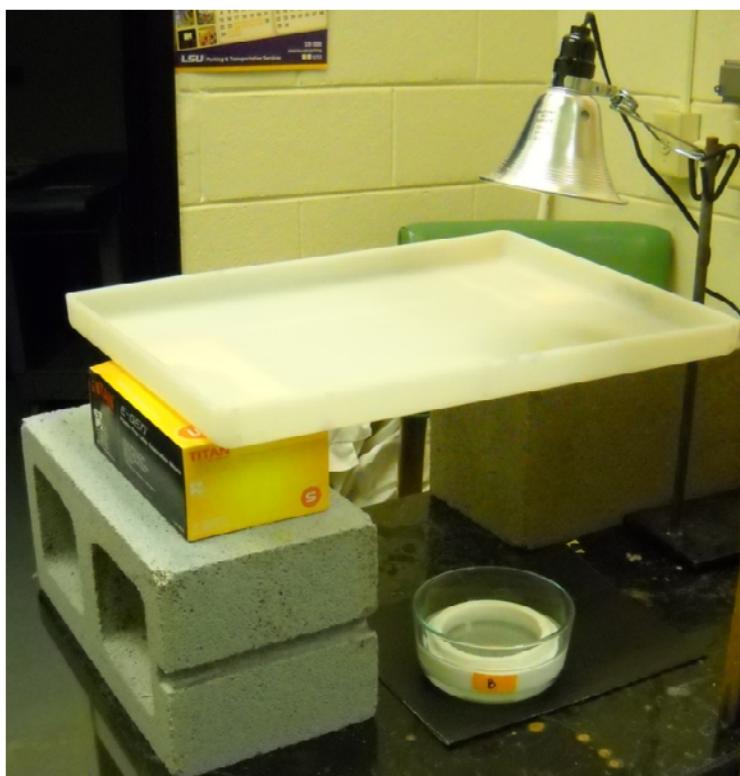
Figure E.1. Set-up for imaging oil slicks indoors.
