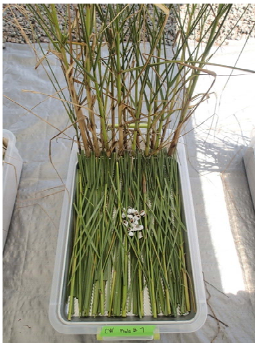
Figure E.1. Control chamber, with horizontal and vertical stalks and no oil.
