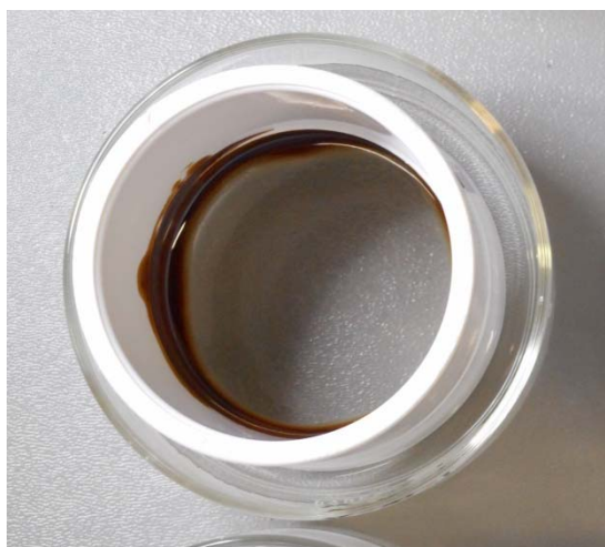
Figure M.1. Top view of the crystallizing dish slick exposure set-up.
