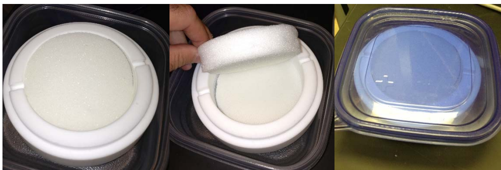
Figure 11.3. Example of plastic container with polyurethane foam used to air-incubate embryos.
