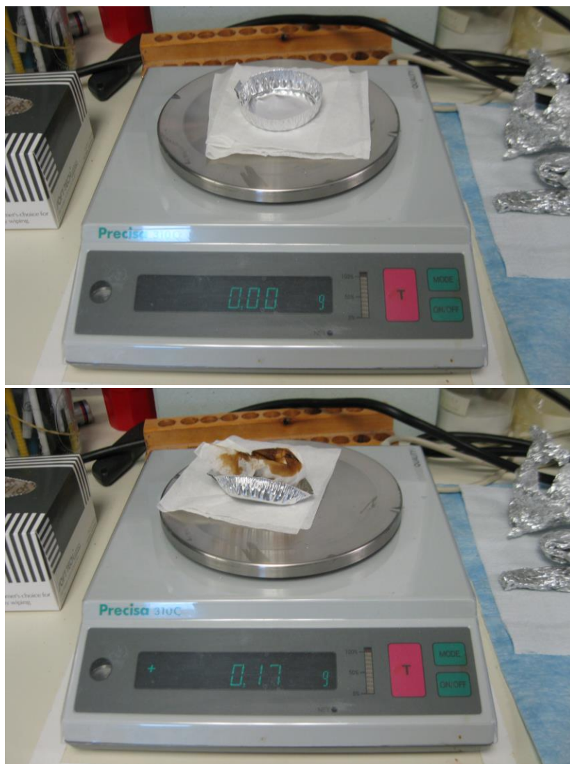
Figure A.2. Taring Kimwipes and aluminum weigh boat and reweighing scraped weigh boat and Kimwipe used to clean spatula.
