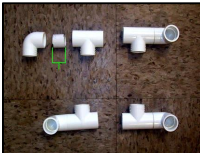
Fig. 95. Construction of carrier corners.
