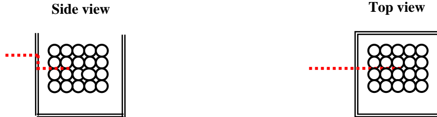
Fig. 62. Styrofoam incubation box showing placement of temperature probe from side view and top view.
