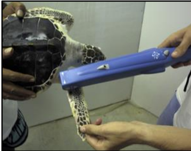
Fig. 90. Proper magnetometer positioning over a flipper for coded wire tag detection (NOAA Fisheries Photo).
