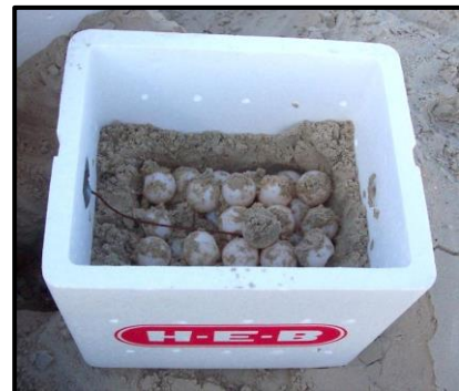
Fig. 60. Insert the thermocouple probe straight into the center of the egg mass.
