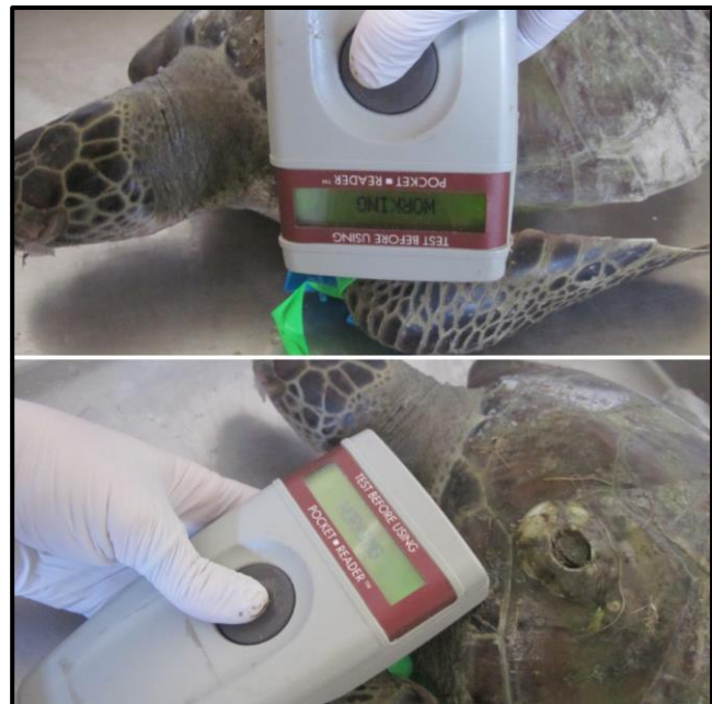
Fig. 39c. Incorrect (top) vs correct (bottom) use of PIT tag reader. In order for tag presence to be detected, the back of the scanner must be pressed flush against the flipper.
